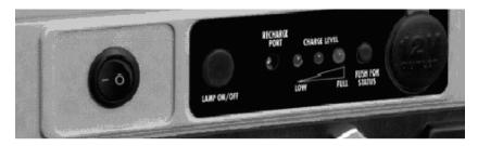
The **VEC270MG** can be recharged from any standard 120 volt AC power source using the supplied AC recharge adapter. The adapter's barrel connector attaches to the recharge port on the side panel.
